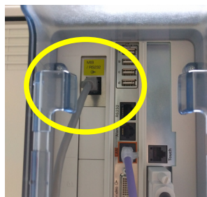
Additional connection from yellow MIB port on the back of the Philips monitor
